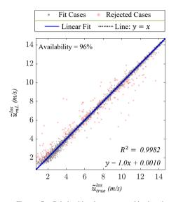
Figure 7. Relationship between machine-learning-predicted spectral median,  $\widetilde{w}_{m,l}^{los}$ , and the true value,  $\widetilde{w}_{true}^{los}$ , from the 13,383 testing cases. The red data indicate predictions with low confidence as explained in Section 32.3.3. Removing these datapoints, which was done before the regression fitting, leaves partial data availability as indicated. Note that the y=x line is mostly obstructed from view by the linear fit line.
