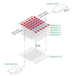
Figure 6. Depiction of the ensemble neural network structure. Note that input and output layers are omitted for clarity.
