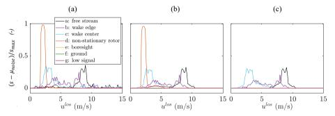
Figure 5. Traces of noise-subtracted and rescaled normalized power spectral density,  $(s - \mu_{noise})/s_{max}$ , versus  $u^{los}$  where  $s_{max} = 2^{16} - 1$ . These cases demonstrate the progression of the primary advanced filtering steps: (a) removal of hard targets; (b) bilateral filtering, thresholding, and isolation of ROI; and (c) combined outlier detection method and low signal quality filter.
