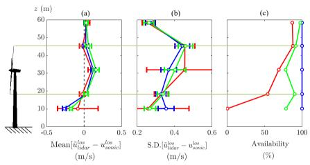
Figure 15. Aggregate results from waked cases for (a) mean error, (b), standard deviation (S.D.) of error, and (c) data availability plotted versus height off the ground. The dimensions of a V27 turbine as used in the experiment are shown for reference. The line colors are: thresholding (—), advanced filtering (—), and machine learning (—).
