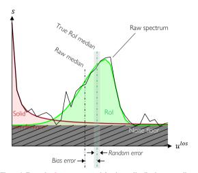
Figure 1. Example of a power spectral density, s, distribution versus line-of-sight velocity,  $u^{los}$ , of a raw CW lidar return illustrating the contamination of the region of interest (RoI) by solid interference and amplitude noise. The raw geometric median contains bias error due to the solid interference as well as random error due to the amplitude noise. Figure adapted from Brown and Herges (2020).
