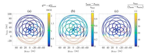
Figure 4. Details of final filtering techniques applied between Figure 3 (b) and (c) using colormaps of the rosette scan pattern: (a) outlier detection from the difference between spectral median line-of-sight velocity,  $\tilde{u}^{los}$ , and smoothed spectral median line-of-sight velocity,  $\tilde{u}^{los}$ , an
