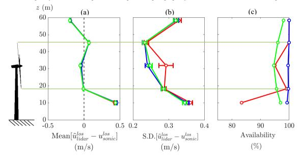
Figure 14. Aggregate results from inflow cases for (a) mean error, (b), standard deviation (S.D.) of error, and (c) data availability plotted versus height off the ground. The dimensions of a V27 turbine as used in the experiment are shown for reference. The line colors are: thresholding (-), advanced filtering (-), and machine learning (-).
