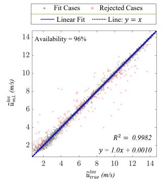
Figure 7. Relationship between machine-learningpredicted spectral median,  $\tilde{u}_{m.l.}^{los}$ , and the true value,  $\tilde{u}_{true}^{los}$ , from the 13,383 testing cases. The red data indicate predictions with low confidence as explained in Section 3.3.3. Removing these datapoints, which was done before the regression fitting, leaves partial data availability as indicated. Note that the y = x line is mostly obstructed from view by the linear fit line.
