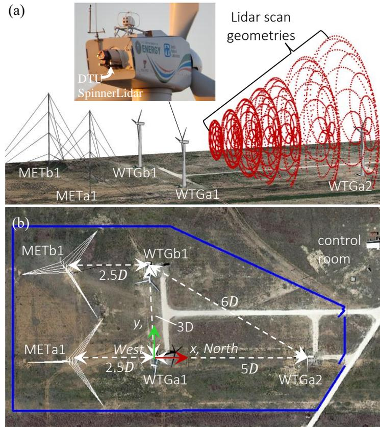
**Figure 2. (a) Rendering of the SWiFT facility in Lubbock, Texas, USA. The nacelle of WTGa1 was outfitted with a rear-mounted DTU SpinnerLidar, which scanned the flow at different focus lengths according to the rosette patterns shown in red. Rendering from Doubrawa et al. (2020). (b) Planform view of the site where  $D = 27$  m. Adapted from Herges and Keyantuo (2019).**
