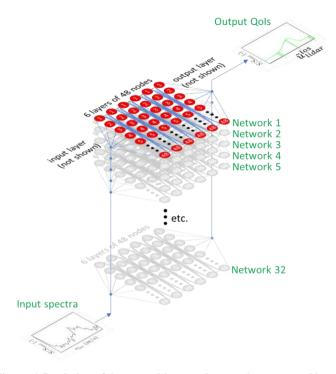
Figure 6. Depiction of the ensemble neural network structure. Note that input and output layers are omitted for clarity.
