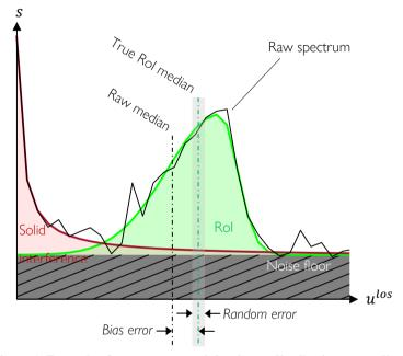
Figure 1. Example of a power spectral density, s, distribution versus lineof-sight velocity,  $u^{los}$ , of a raw CW lidar return illustrating the contamination of the region of interest (RoI) by solid interference and amplitude noise. The raw geometric median contains bias error due to the solid interference as well as random error due to the amplitude noise. Figure adapted from Brown and Herges (2020).
