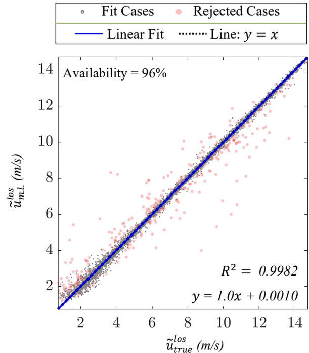
**Figure 7. Relationship between machine-learning-predicted spectral median,  $\tilde{u}_{m.l.}^{los}$ , and the true value,  $\tilde{u}_{true}^{los}$ , from the 13,383 testing cases. The red data indicate predictions with low confidence as explained in Section 3.3.3. Removing these datapoints, which was done before the regression fitting, leaves partial data availability as indicated. Note that the  $y = x$  line is mostly obstructed from view by the linear fit line.**
