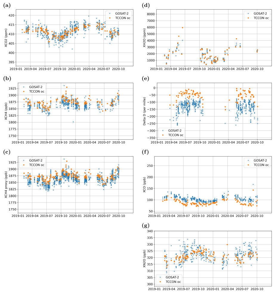
Figure 16. Example time series of TCCON and GOSAT-2 FOCAL data at Lamont (station code oc). (a) XCO 2 . (b) XCH 4 full physics product. (c) XCH 4 proxy product. (d) XH 2 O. (e) δD. (f) XCO. (g) XN 2 O.
