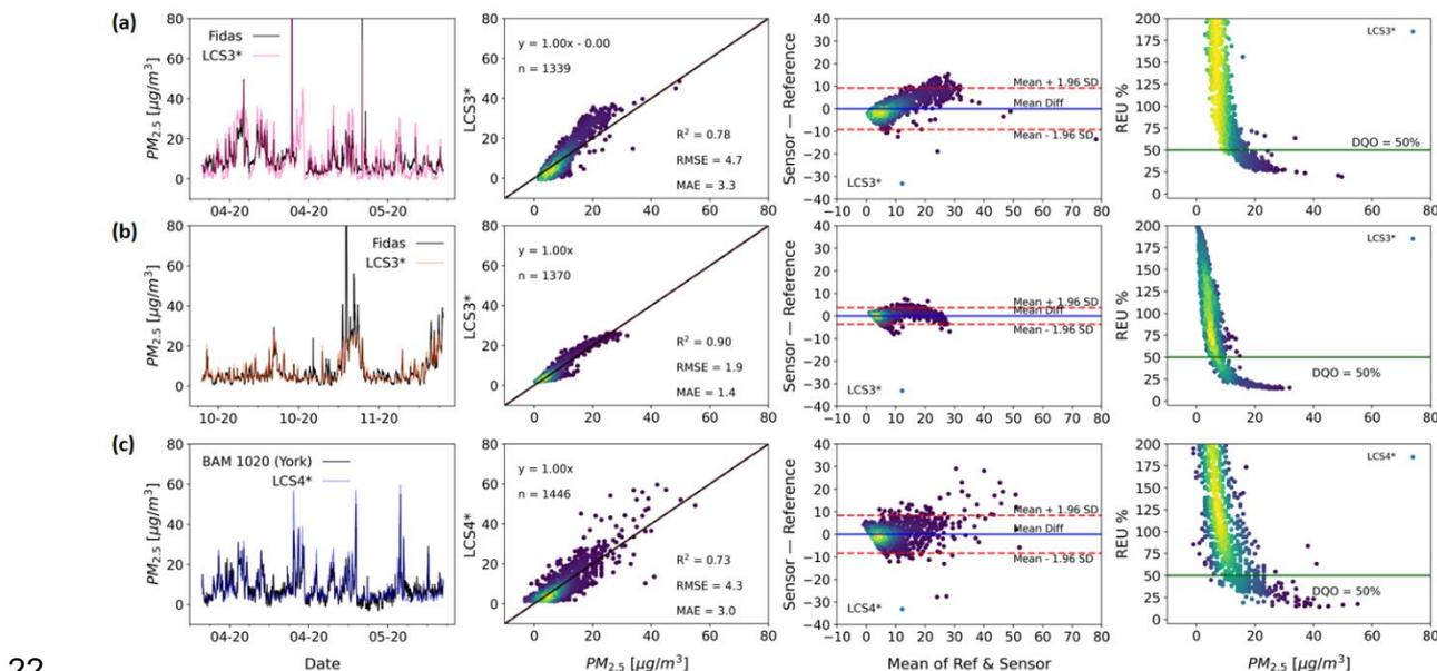
22 **Figure S2. Two bias corrected LCS systems (LCS3 & LCS4, same brand) measuring PM<sub>2.5</sub> (Time res 1 h). While LCS3**
