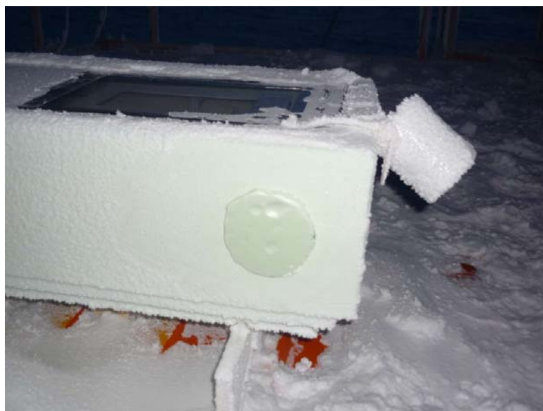
214 Fig. 6: ICECAMERA at -70°C, Concordia station winter: the DS is free of frost
