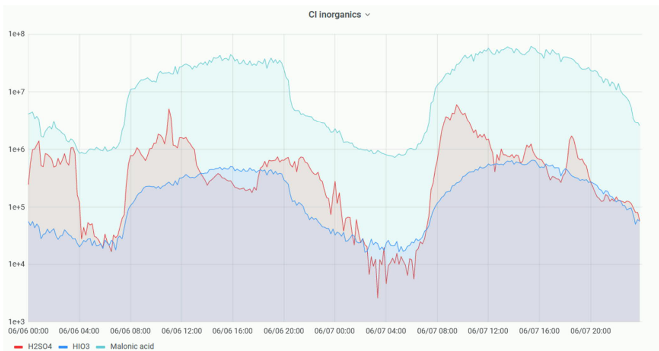
Figure 7. CI-API-TOF on-line inorganic acid concentrations (sulphuric acid shown in red, iodic acid in blue and malonic acid in cyan) measured at the SMEAR Estonia station during 6.6.2021–7.6.2021. The formation of all three acids is initiated by solar radiation and formation of OH-radicals, however the precursor gases are different, \text{SO}_2 , \text{I}_2 , and a wide variety of volatile organic compounds, respectively.
