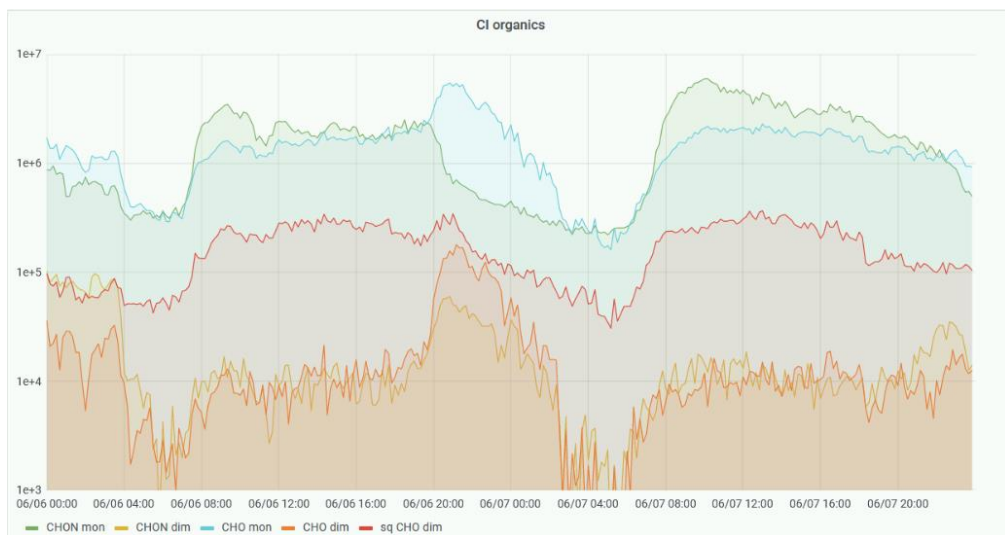
Figure 5. Chemical Ionization Atmospheric Pressure interface Time-Of-Flight (CI-APiTOF) mass spectrometer on-line data of highly oxidized organic molecule (HOM) concentrations measured at the SMEAR Estonia station during 6.6.2021 - 7.6.2021. In the legend capital letters denote chemical elements present in the molecule, “mon” denotes monomers and “dim” dimers, prefix “sq” denotes that HOM are formed from sesquiterpenes. The others are formed from monoterpenes. Both sesquiterpenes and monoterpenes are volatile compounds emitted by vegetation. Inorganic acid concentrations could be presented similarly or even added to the plot by the user as needed. The processing done by SMEARcore allows showing these concentrations instead of raw counts from the instrument.
