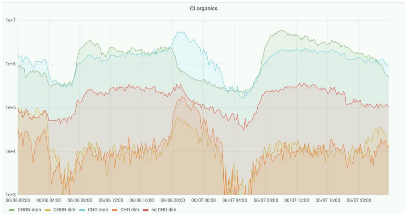
295 Figure 5. Chemical Ionization Atmospheric Pressure interface Time-Of-Flight (CI-APiTOF) mass spectrometer on-line data of highly oxidized organic molecule (HOM) concentrations measured at the SMEAR Estonia station during 6.6.2021 - 7.6.2021. In the legend capital letters denote chemical elements present in the molecule, “mon” denotes monomers and “dim” dimers, prefix “sq” denotes that HOM are formed from sesquiterpenes. The others are formed from monoterpenes. Both sesquiterpenes and monoterpenes are volatile compounds emitted by vegetation. Inorganic acid concentrations could be presented similarly.
