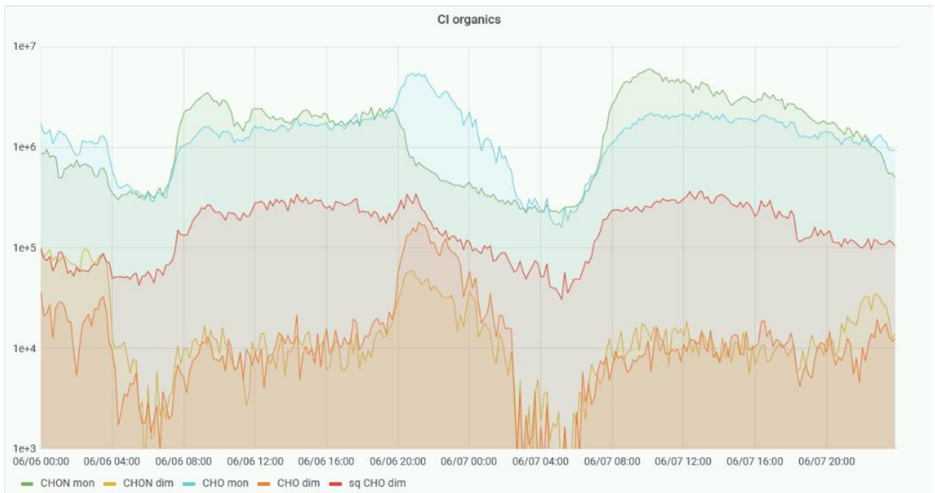
Figure 5. Chemical Ionization Atmospheric Pressure interface Time-Of-Flight (CI-APiTOF) mass spectrometer on-line data of highly oxidized organic molecule (HOM) concentrations measured at the SMEAR Estonia station during 6.6.2021 - 7.6.2021. In the legend capital letters denote chemical elements present in the molecule, “mon” denotes monomers and “dim” dimers, prefix “sq” denotes that HOM are formed from sesquiterpenes. The others are formed from monoterpenes. Both sesquiterpenes and monoterpenes are volatile compounds emitted by vegetation. Inorganic acid concentrations could be presented similarly or even added to the plot by the user as needed. The processing done by SMEARcore allows showing these concentrations instead of raw counts from the instrument.
