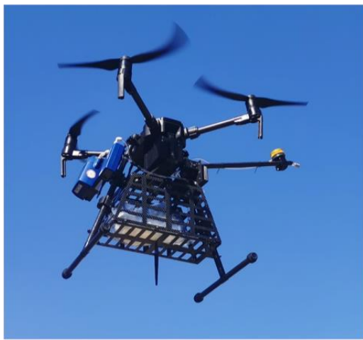
Figure 1: Photo and schematic representation of the gas sampling system (blue) and aerosol measurement system (black) as installed on the DJI Matrice 200 UAS.
