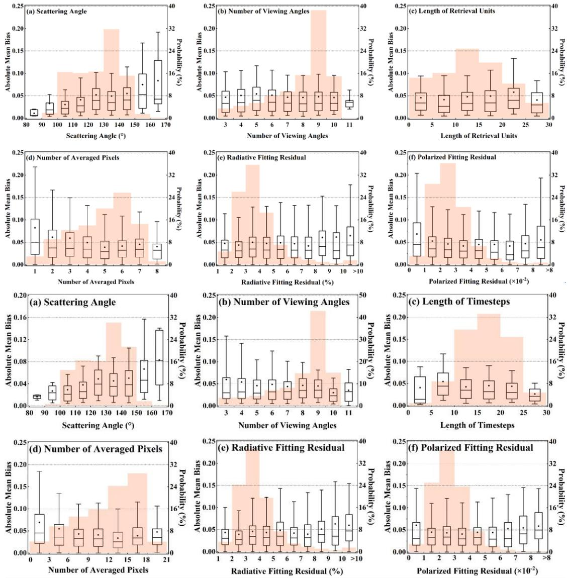
**Figure 3.** Influencing factors of AOD retrieval performance of DPC based on the GRASP/Model: (a) SCA; (b) number of viewing angles; (c) length of timesteps; (d) number of averaged pixels; (e) non-polarized fitting residual; (f) polarized fitting residual. Orange shadows in the background represents the probability distribution of the samples.
