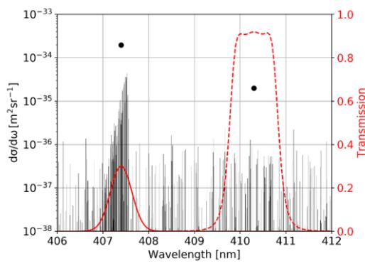
**Figure 4.** Water vapor Raman cross-section spectrum (black) is shown together with the transmission of the water vapor channel filter (red) and the new fluorescence monitoring channel filter (dashed, red). The total water vapor Raman cross-section for these two channels as the result of integrating the product of the Raman cross-section spectrum with the filter transmission of each channel between 406 nm and 412 nm is also shown (dots, black).
