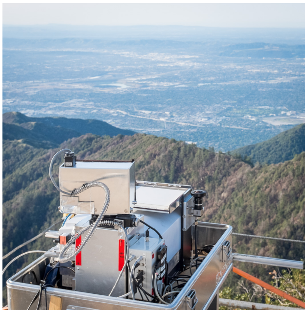
Figure 1. The EM27/SCA instrument on top of Mt. Wilson overlooking the Los Angeles Basin. The pointing mirrors are located inside the upper metal protective housing, shielding them from direct sun light. The depicted viewing direction points away from the observer into the basin. The Lambertian reflector plate is mounted on top of the instrument's main body. The context camera is attached on the right.
