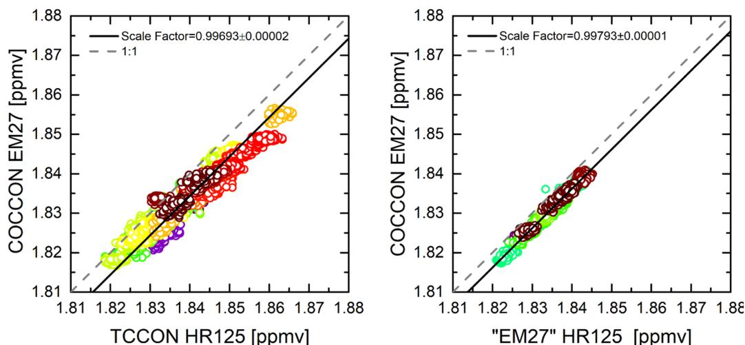
Figure 2. Comparison between the COCCON EM27/SUN and high-resolution (HR) IFS 125 retrievals for CO<sub>2</sub> and CH<sub>4</sub> at the Izaña Observatory. The HR IFS 125 observations are taken using the TCCON (TCCON HR12) and COCCON EM27/SUN measurement settings (EM27 HR125).
