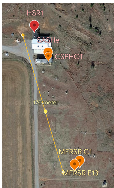
100 Figure 1: Map of the instruments at the ARM SGP site. The HSR1 is indicated by a red marker and all other instruments are shown with an orange marker. The instrument names are labelled near their respective markers. The yellow line indicates a distance of 170 m for scale.
