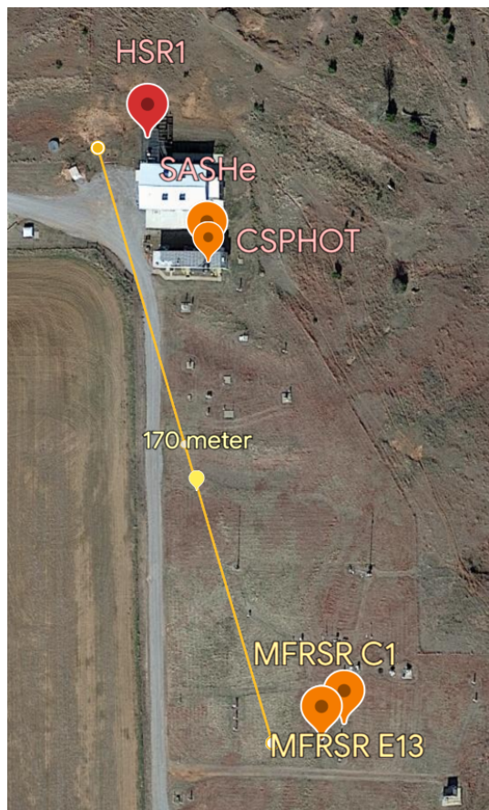
Figure 1: Map of the instruments at the ARM SGP site. The HSR1 is indicated by a red marker and all other instruments are shown with an orange marker. The instrument names are labelled near their respective markers. The yellow line indicates a distance of 170 m for scale.
