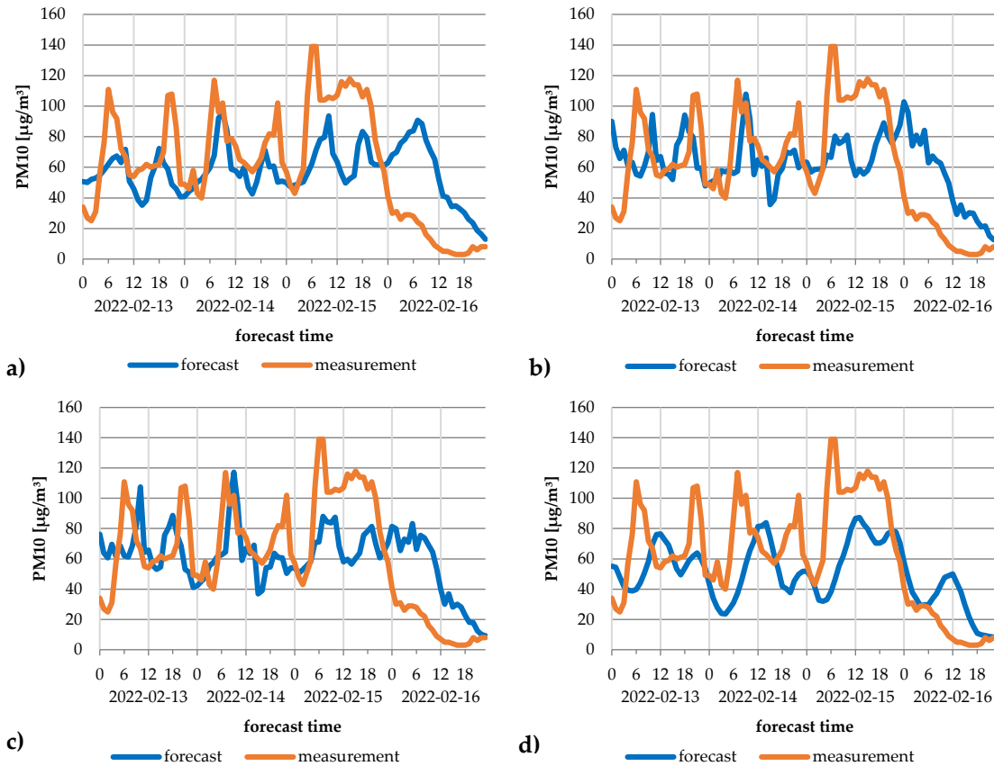
Figure 12. Measurements and forecasts for 13–16 February 2022: a) forecast without SODAR data; b) forecast predicted by regression without hours; c) full regression forecast; d) search method forecast.
