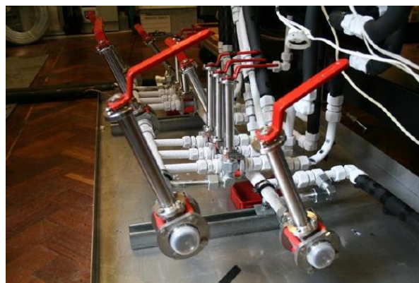
Figure S1(b): Inlet manifold to divert the fluid from the thermostat into 4 separate circulation pathways.
