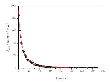
**Figure 4:** Typical HO<sub>2</sub> decay recorded at 293 K and 1000 mbar air. The red line is the fit to the data from equation (E5) giving  $C_{\text{HO2, 293 K}} = (4.17 \pm 1.66) \times 10^{-8} \text{ counts cm}^3 \text{ molecule}^{-1} \text{ mW}^{-1} \text{ s}^{-1}$
