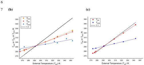
**Figure 2:** (a) Schematic of FAGE Cell showing locations of thermocouples. (b) Internal cell temperatures ( $T_{\rm OH}$  or  $T_{\rm HO2}$ ) and inlet temperatures ( $T_{\rm inlet}$ ) plotted as a function of the external temperature ( $T_{\rm ext}$ ), when sampling air at 293 K from the calibration flowtube. (c) Internal temperatures as a function of the external temperature when either sampling temperature controlled air from the calibration flowtube or sampling from the HIRAC chamber.
