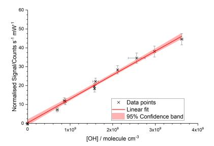
Figure 1: Typical room temperature calibration plot from the conventional water photolysis, flow tube method. The total flow rate was 40 slm, with [H<sub>2</sub>O] = 1600 ppmv, the laser power was 9.65 mW and the OH cell was at a pressure of 2.6 Torr. Gradient =  $(1.266 \pm 0.034) \times 10^{-8}$  counts s<sup>-1</sup> mW<sup>-1</sup> cm<sup>3</sup> molecule<sup>-1</sup>, intercept =  $0.28 \pm 0.74$  counts s<sup>-1</sup> mW<sup>-1</sup>. Errors are  $2\sigma$ .
