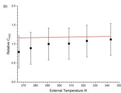
**Figure 5:** Temperature dependence of the calibration factors ( $C_{\text{HOX}}$ ) as a function of the external temperature with HOx being delivered from the calibration flow tube at a constant temperature. (a)  $C_{\text{OH,obs}}$ , slope =  $(0.0023 \pm 0.0007) \text{ K}^{-1}$ . (b)  $C_{\text{HO2,obs}}$ , slope =  $(0.0005 \pm 0.0031) \text{ K}^{-1}$ . Errors are  $2\sigma$ .
