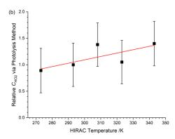
**Figure 7**: Temperature dependence of  $C_{\text{HOx,obs}}$  relative to values at 293 K. (a) Relative  $C_{\text{OH,obs}}$  from the HC decay method. Slope =  $(0.0038 \pm 0.0007)$  K<sup>-1</sup> (b) Relative  $C_{\text{HO2,obs}}$  from the HCHO photolysis method. Slope =  $(0.0064 \pm 0.0034)$  K<sup>-1</sup>. Errors are  $2\sigma$ .
