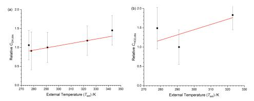
**Figure 6:** Temperature dependence of the calibration factors ( $C_{\text{HOx,obs}}$ ) as a function of the external temperature with HOx being delivered from the calibration flow tube at the external temperature. (a)  $C_{\text{OH,obs}}$ , slope =  $(0.0059 \pm 0.0015) \text{ K}^{-1}$ . (b)  $C_{\text{HO2,obs}}$ , slope =  $(0.014 \pm 0.013) \text{ K}^{-1}$ .
