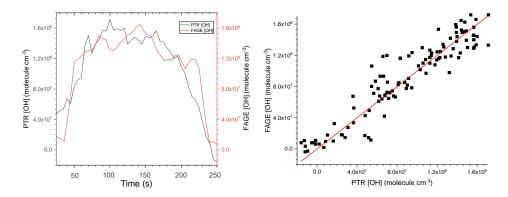
**Figure 3:** a) Time series of [OH] derived from FAGE measurements and from mass spectrometric measurements of cyclohexane removal recorded following  $H_2O_2$  photolysis at 293 K and 1000 mbar air. b) Resultant scatter plot where the gradient,  $0.998 \pm 0.016$  (2 $\sigma$ ) gives  $C_{\text{rel}}$  for the FAGE apparatus at 293 K for this experiment. The average gradient at 293 K is  $1.034 \pm 0.0068$  from five experiments.
