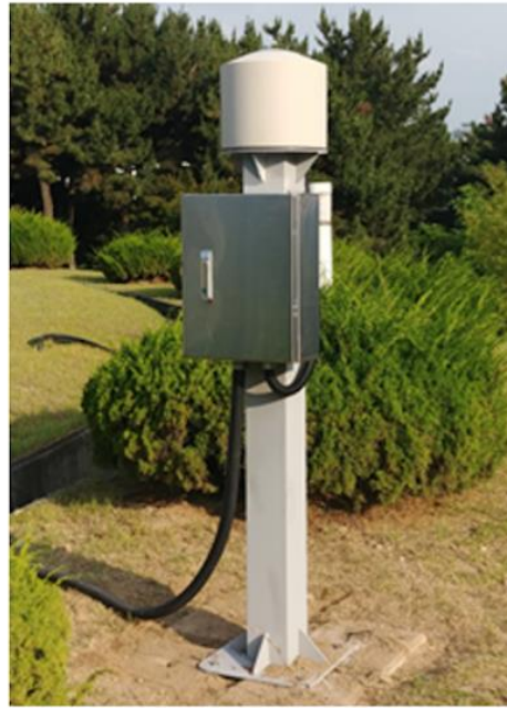
Figure 1: Appearance of automatic cloud observation system (ACOS) (a) and installation environment (b) (Kim and Cha, 2020).
