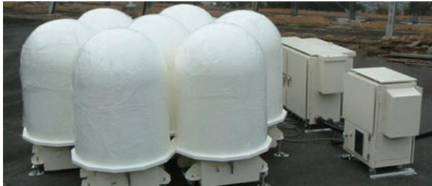
Figure 1. WPR LQ-7 Luneberg Lens antenna array.
