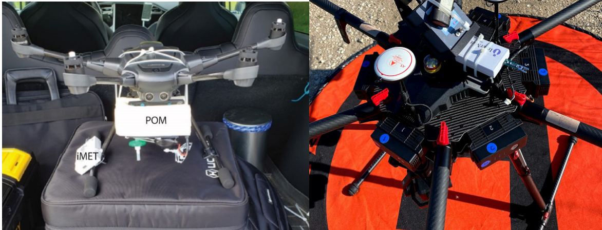
Figure 2. a) Typhoon H UAS with mounted POM and iMet-XQ2 as flown during CHEESEHEAD-19 in 2019. POM was housed in foam for vibration dampening. b) Top mounted iMet-XQ2 and POM on a DJI M600 as flown in Sept. 2020 for WiscoDISCO20. The inlet to the POM is held up with a bracket to hold the inlet filter assembly (blue and white).
