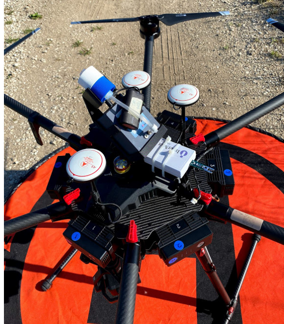
Figure S2. Top mounted iMet-XQ2 and POM on a DJI M600. The inlet to the POM is held up with a bracket to hold the inlet filter assembly (blue and white).
