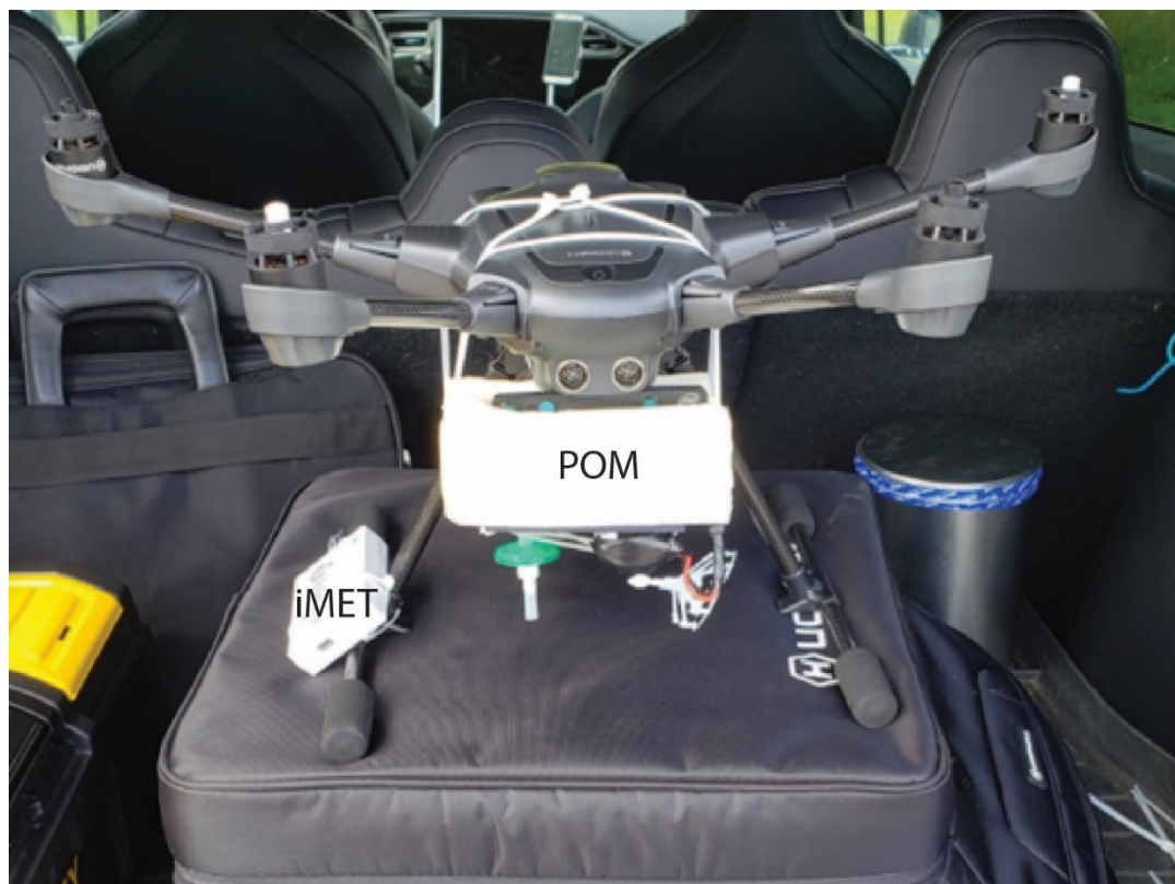
Figure S1. Typhoon H UAS with mounted POM and iMet-XQ2 as flown during CHEESEHEAD-19 in 2019. POM was housed in foam for vibration dampening.
