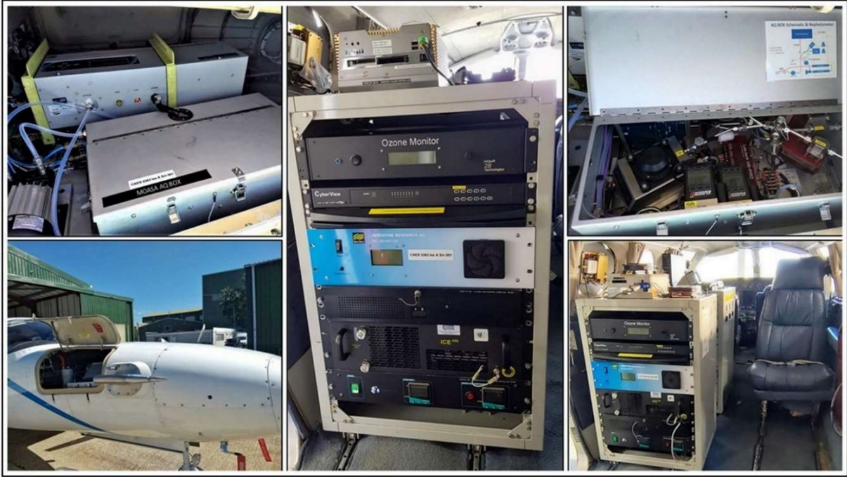
160 Figure 2: Clockwise starting top left: the AQ box (foreground) and nephelometer (background) in the MOASA nose bay; the aft instrumented rack housing the O 3 , NO 2 and aerosol LIDAR control system; inside the AQ box; inside the cabin looking forward; the Brechtel isokinetic air sample inlet and nose bay of the MOASA.
