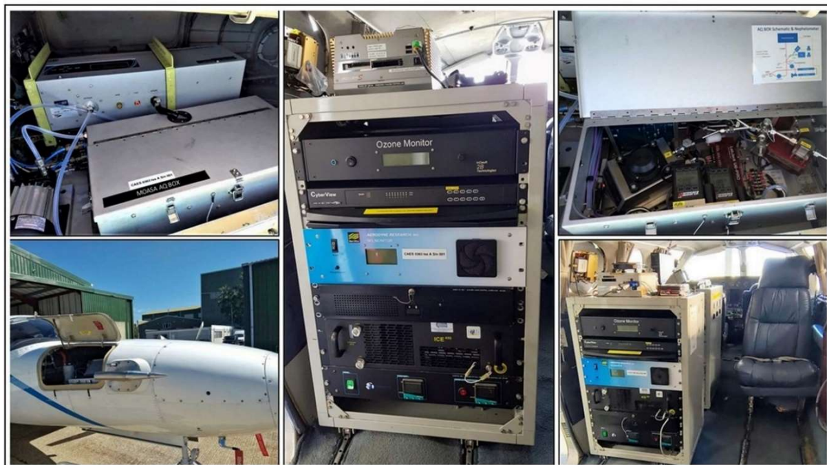
Figure 1: The Met Office Atmospheric Survey Aircraft with instrumentation. Image courtesy Debbie O'Sullivan, Met Office, 2021.
