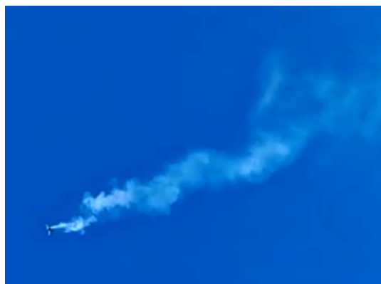
Figure 2. Image of the seeding UAV hovering at 150 m above ground while an attached flare is burning (out-of-cloud). The photo contrast was enhanced to make the plume more visible.
