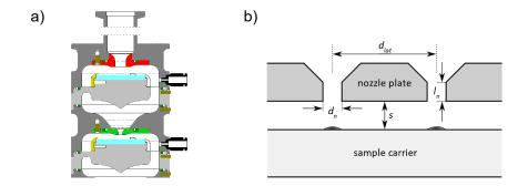
95 Figure 1: a) Schematic of the first two impactor stages, with an upper body (dark grey) accommodating the nozzle module (red and green) and a lower body (light grey) accommodating the sample carrier (light blue).
