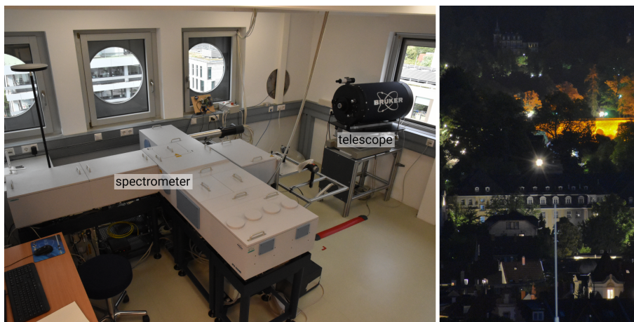
Figure 2. Left: Overview of the roof-top observatory of the IUP with the IFS 125HR spectrometer in the center, as well as the telescope pointing out a window. Right: View along the light path at night, with the reflector array on top of the OPI shining bright in the center of the picture.
