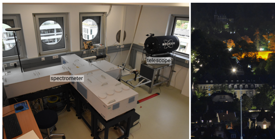
Figure 2. Left: Overview of the roof-top observatory of the IUP with the IFS 125HR spectrometer in the center, as well as the telescope pointing out a window. Right: View along the light path at night, with the reflector array on top of the OPI shining brightly in the center of the picture.
