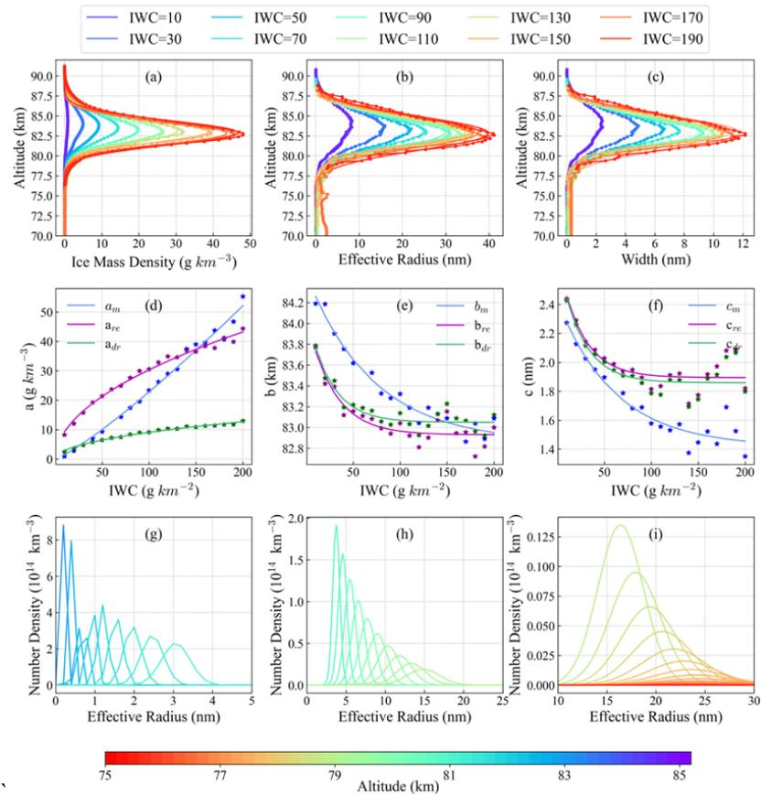
335 **Figure 4: (a)-(f) Data fitting of the ice mass content, effective radius, and particle size spectrum width. (g)-(i) Scale spectrum distribution at different heights (75–85 km) when  $\text{IWC} = 100 \text{ g km}^{-2}$ .**
