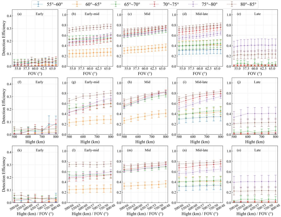
**Figure 11: (a)-(e) Variation in detection efficiency with the FOV at different latitudes during different periods; (f)-(j) Variation in detection efficiency with the satellite altitude at different latitudes during different periods; (k)-(o) variation in detection efficiency with simultaneous changes in the FOV and satellite altitude at different latitudes during different periods.**
