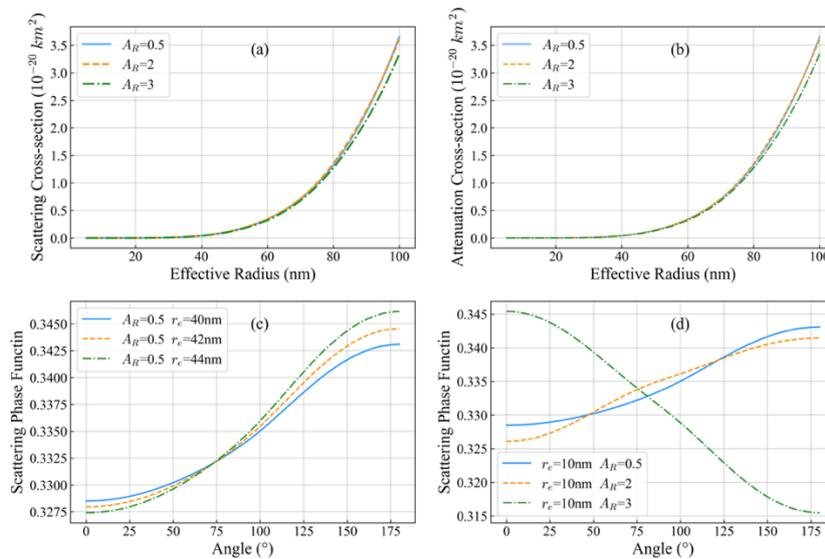
**Figure 3:** Panels (a) and (b) shows the scattering and extinction cross-section regarding particle effective radius ( $r_e$ ) respectively at different axis ratio ( $A_R = 0.5, 2, 3$ ). Panel (c) denotes the scattering phase function at WL = 265 nm for different  $r_e$ , while Panel (d) denotes the scattering phase function at  $r_e = 10 \text{ nm}$  for different  $A_R$ .
