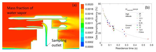
Figure 6: (a) contour plot of mass fraction of water vapor of the inlet for 25mm restrictor with freestream velocity of 180m/s, freestream turbulence intensity of 3%, and angle of attack of 3°. (b) correlation between residence time inside the sampling tube and the overall gas sampling efficiency at the sampling outlet for all restrictors under different altitudes, freestream velocities and sampling velocities.
