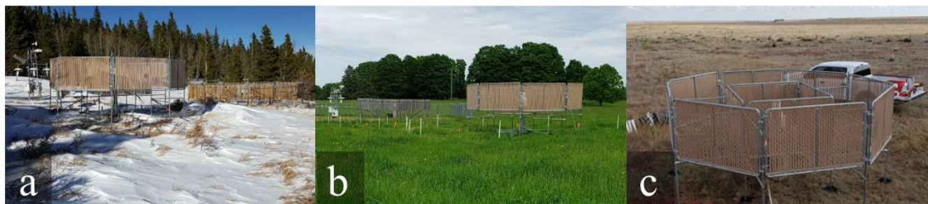
Fig. 53: Photos of Low Porosity Double Fence (LPDF) shields installed at the Boulder, CO (a), Chatham, MI Marshall, CO (b), and Marshall, CO Chatham, MI (c) sites.
