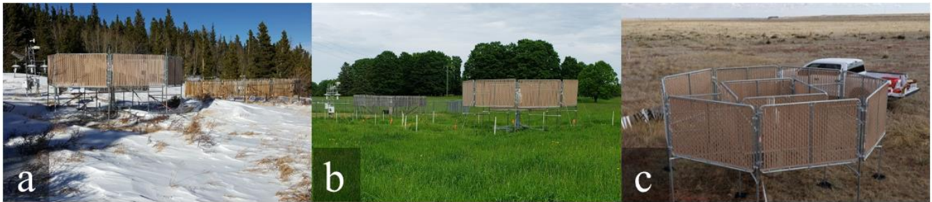
445 Fig. 5: Photos of Low Porosity Double Fence (LPDF) shields installed at the Boulder, CO (a), Chatham, MI (b), and Marshall, CO (c) sites.
