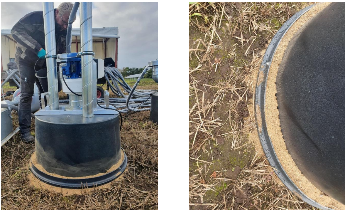
Figure S4. Dynamic flux chamber in the field with sand sealing at the soil surface.
