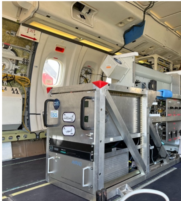
Figure S3 Photo of the A2S2 configured as part of the AVIRAD system onboard the ATR-42
