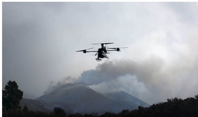
Figure 1. A Dragonfly UAS returning from a CO 2 sample mission during the November 2021 eruption of Tajogaite volcano. The large volcanic ash plume is visible in the background and contains an invisible CO 2 plume, which was the mapping target of this drone.
