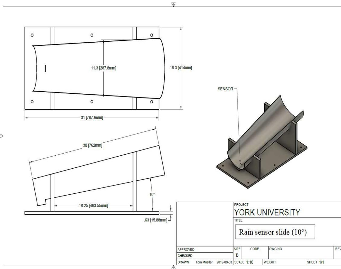
**Figure S8.** Design and dimensions (in mm) of the mounting chute for the rain sensor. The chute slope is fixed at an optimized angle of 10°, that maintains water on the surface of the sensor throughout a rain event but allows excess water to flow over the sensor when necessary. We also tested 15° and 20° through manual observation but found that rainwater would flow over the sensor too rapidly – limiting or even preventing detection of wet deposition events.
