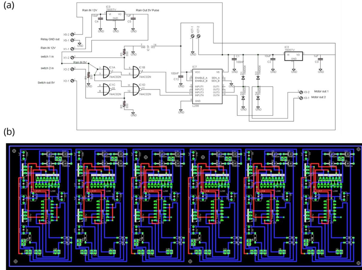
**Figure S9.** Technical schematics for all printed circuit board components required to control (a) one precipitation collector with all components and connections to chips indicated and (b) a complete six-unit array composed of replicate layouts.
