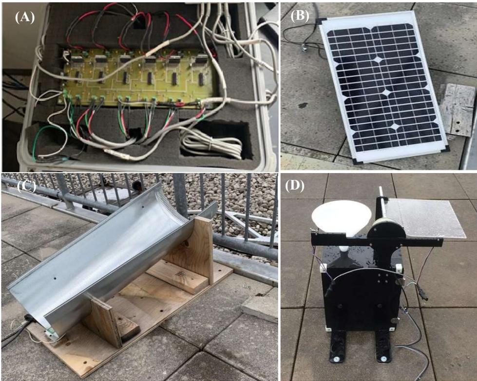
**Figure S1.** Automated precipitation array stationed at the Air Quality Research Station, York University, Toronto, consisting of: (A) weather-proofed control board, (B) 40 W solar panel, (C) rain sensor, and enhanced sensitivity chute, and (D) an automated collection unit fixed to concrete with lag sleeves and bolts during a rain event.
