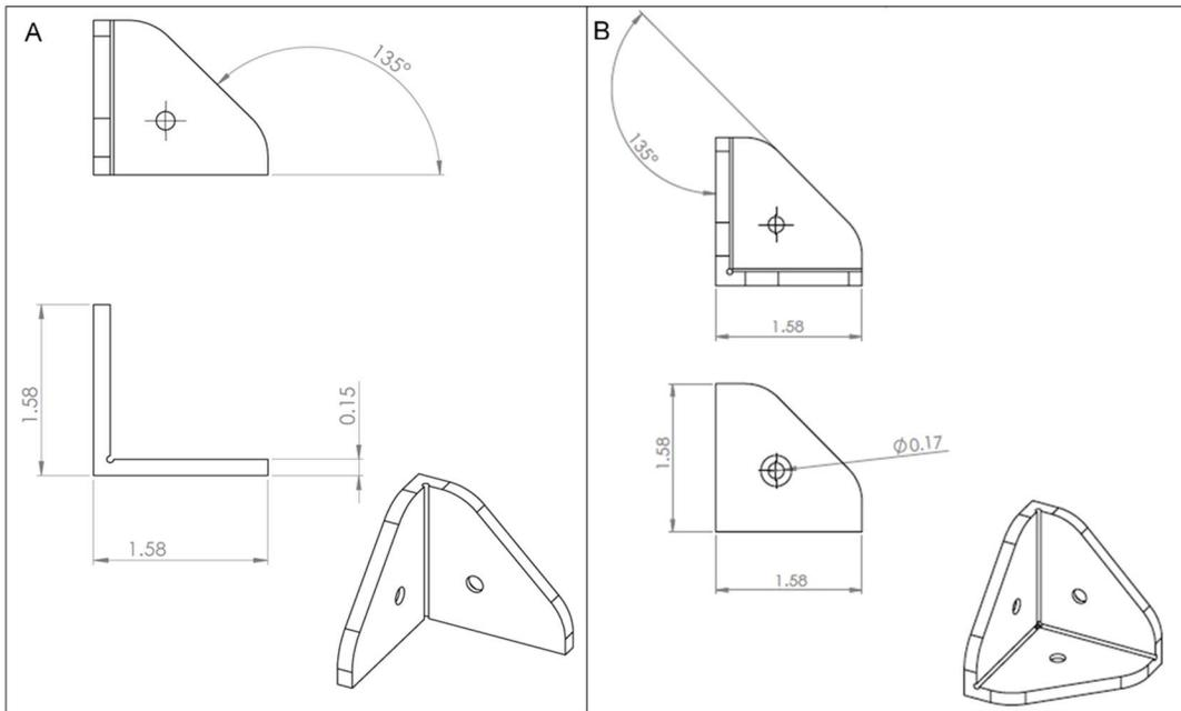
**Figure S4.** Dimensions (in millimeters) of 3D printed corner options: **(A)** double corner to affix panels adjoining the door and **(B)** multi corner used to secure three panels throughout the remainder of the collection unit.
