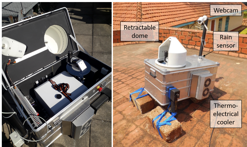
Figure 2. Left: internal view of the EM27/SUN spectrometer and solar tracker housed within the TU Munich enclosure system; Right: the enclosure system in operation at NaFIRRI, with the two car-jacks used to tilt the system to enable tracking of the sun at very high solar zenith angles (see text in Section 2.2). The bricks attached to the car-jacks anchor the enclosure down in case of strong winds.
