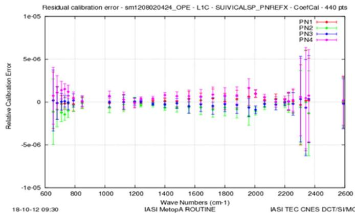
Figure 2 : Residual inter-pixel relative spectral calibration ( $\Delta\nu/\nu$ ) for the orbit of 2012/08/02 04h24 (Jacquette et al., 2013)
