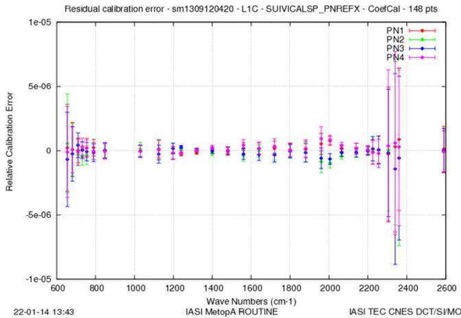
Figure 3 : Residual inter-pixel relative spectral calibration ( $\Delta v/v$ ) for the orbit of 2013/09/12 04h21 (IASI quarterly performance report from 2013/09/01 to 2013/11/30)
