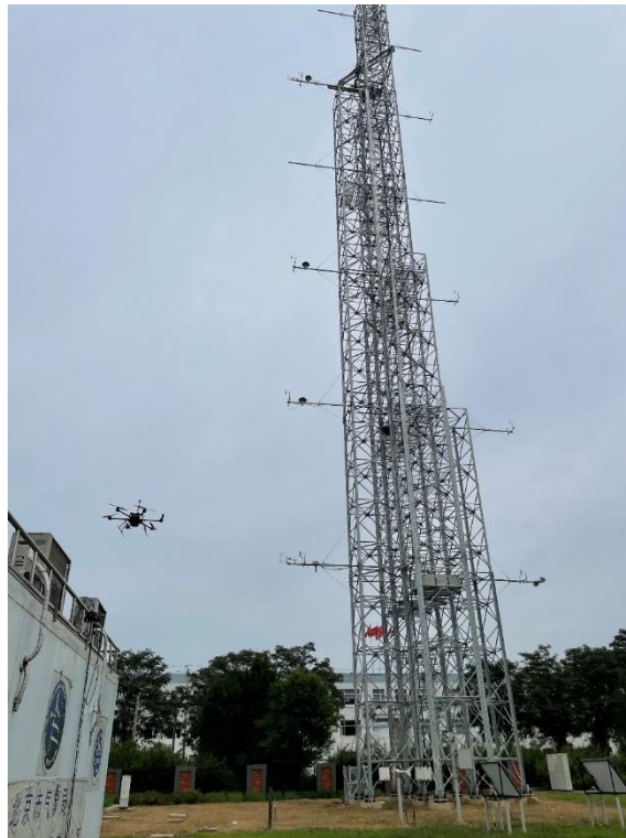
29 Figure S2: Comparison between UAV-based and Tower-based wind speed measurements.
