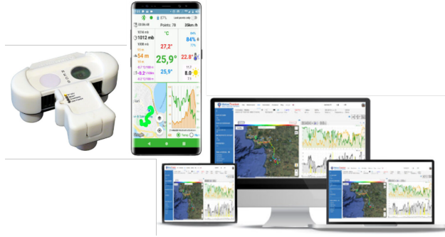
Figure 1. The MT and its components: left to right, the mini-weather station, the mobile application, and the web platform. Collaged from https://meteotracker.com/ (accessed on July 2022).
