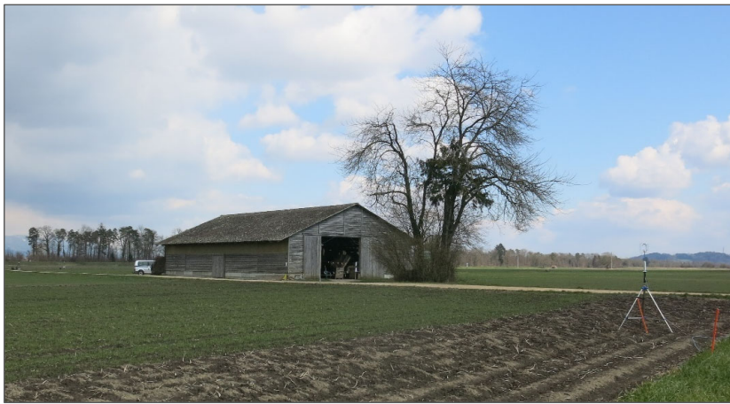
Fig. 1. Barn used for the CH 4 release experiment and the adjacent tree. In the background a river dam with trees on it is visible. The photo was taken from the southwest side of the barn. In the foreground is a 3D ultrasonic anemometer (UA-50m-2.0h).
