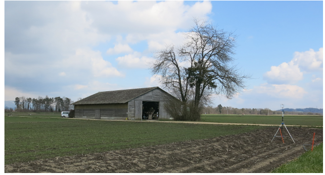
Figure 1. Barn used for the \text{CH}_4 release experiment and the adjacent tree. In the background, a river dam with trees on it is visible. The photo was taken from the southwest side of the barn. In the foreground is a 3D ultrasonic anemometer (UA-2.0h).
