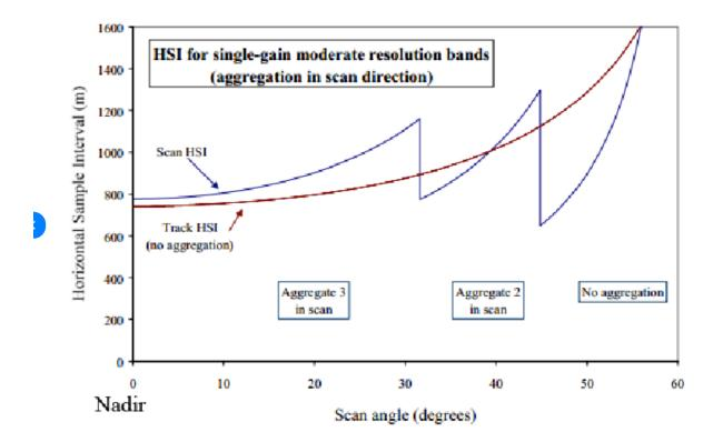
Horizontal sample interval chart shows how the growth of VIIRS M-band ground field of view from nadir to edge of scan is constrained by switching the number of pixels that are aggregated [12]. In aggregation zone 1, from nadir to 31.72 degrees, the signal from three pixels are averaged. In aggregation zone two, the signal from two pixels are averaged. In aggregation zone three, signal from a single pixel is recorded.
