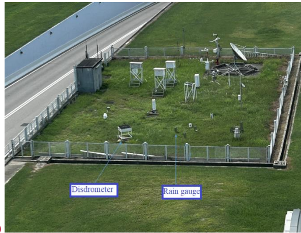
Figure 1: (a) Location of the field test site within the Hong Kong International Airport, (R1E indicates the wind sensor) and (b) picture of the installed rain gauge and 2DVD within the field test site.
