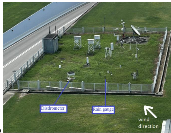
Figure 1: (a) Location of the field test site within the Hong Kong International Airport, (RIE indicates the wind sensor) and (b) picture of the installed rain gauge and 2DVD within the field test site, the white arrow indicates the prevailing wind direction (about 100 degrees).
