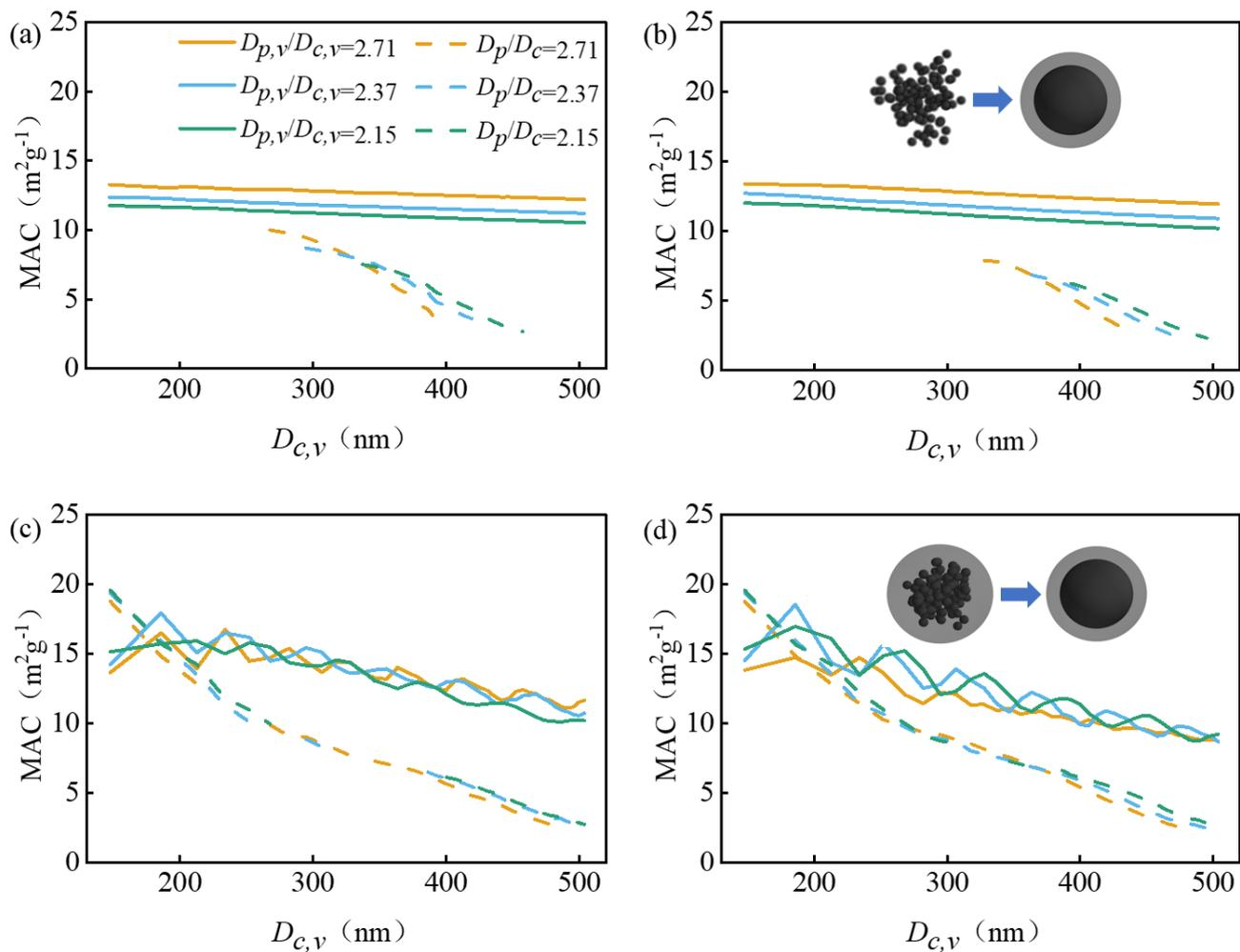
305 **Figure 6.** Differences in mass absorption cross-section (MAC) between fractal particle model (solid lines) and core-shell model (dashed lines) at 532 nm. **(a)** Closed-cell model with  $D_f = 2.40$ ; **(b)** Closed-cell model with  $D_f = 2.60$ ; **(c)** Coated-aggregate model with  $D_f = 2.60$ ; **(d)** Coated-aggregate model with  $D_f = 2.80$ .
