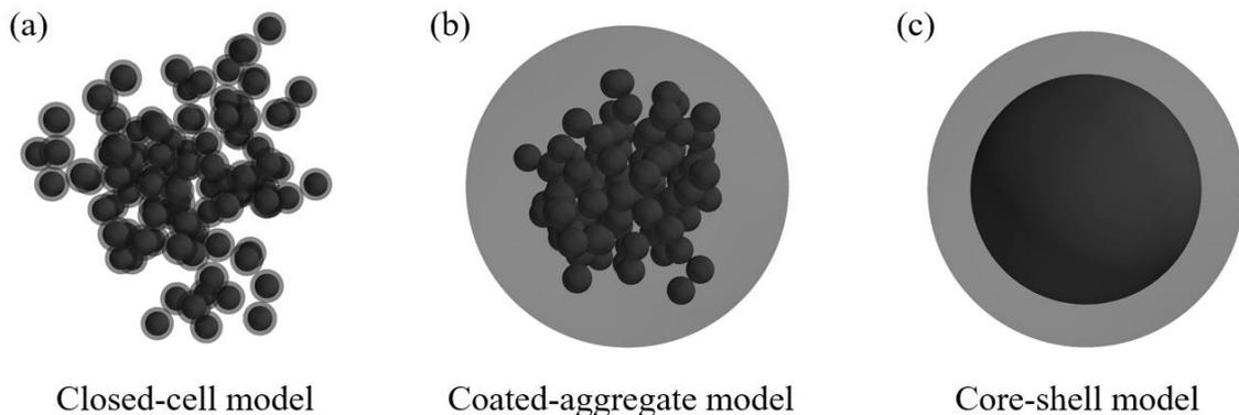
**Figure 1.** Geometries of fractal BC aggregate model with  $N_s=100$  and core-shell model. **(a)** Closed-cell model with  $D_f=2.4$  and  $V_f=0.40$ . **(b)** Coated-aggregate model with  $D_f=2.6$  and  $V_f=0.10$ . **(c)** Core-shell model with  $V_f=0.40$ .
