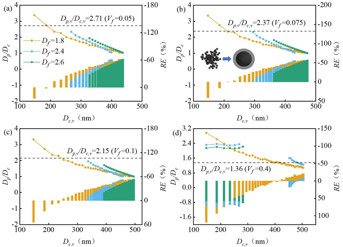
**Figure 3.** Retrieved mixing state ( $D_p/D_c$ ) and relative error ( $RE$ ) as functions of volume equivalent diameter ( $D_{c,v}$ ) for thinly coated BC particles with different  $D_f$  and  $D_{p,v}/D_{c,v}$ . The colored lines stand for retrieved  $D_p/D_c$  and the colored bars stand for  $RE$ .
