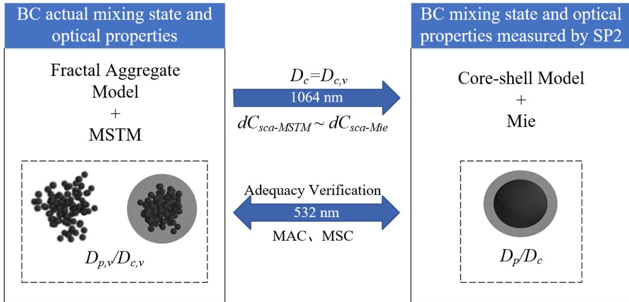
200 **Figure 2.** Schematic overview of the methodology of both the BC mixing state retrieval, and the verification of optical property at 532 nm predicted based on SP2 retrieval results.
