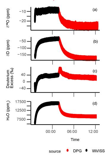
**Figure S7.** Full sweepout curve of 100 foot (30.48 m) Bev-A-Line XX for  $\delta^{18}O$  (a),  $\delta D$  (b), D-excess (c), and H<sub>2</sub>O (d) in both depleted-to-enriched (black points) and enriched-to-depleted (red points) directions. Bev-A-Line XX takes approximately 6 hours to fully equilibrate in either direction of the switch. The time to equilibration is longer in the enriched-to-depleted direction.
