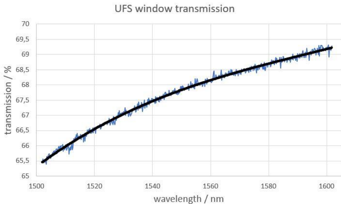
Figure R1.2: Transmission of the laboratory window. The temperature retrieval depends on the line ratio of emission lines at different wavelengths. Any optical element that exhibits a slope in spectral transmissivity (or reflectivity) can influence the accuracy of the retrieval. The lab window is often overlooked in this context, because it is not always easy to calibrate. Also, it is exposed to environmental conditions with the potential to alter its properties. No such changes have been observed so far at UFS.
