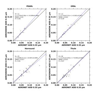
**Figure 4.** Validation of monthly mean AEROSNOW retrieved AOD colocated with monthly mean AERONET observation AOD obtained over PEARL, OPAL, Hornsund, and Thule stations. The linear regression lines are shown as blue dashed line.
